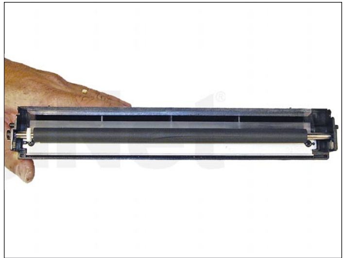
32. Install the PCR by sliding the long shaft side through the non-contact side. Bring it back to fit into the contact side.
