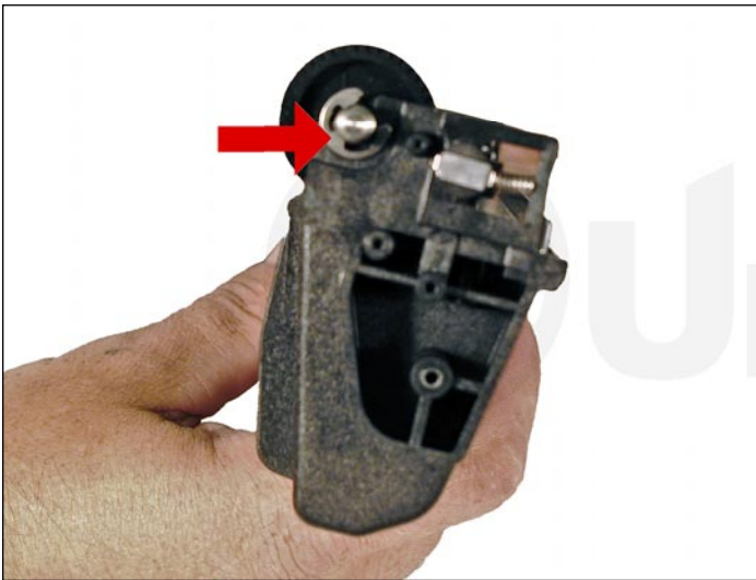
23. On the waste hopper, remove the E-ring from the drum axle.
