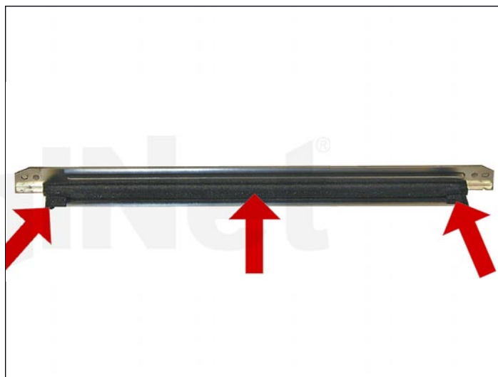
16. Clean out any remaining toner from the hopper.
