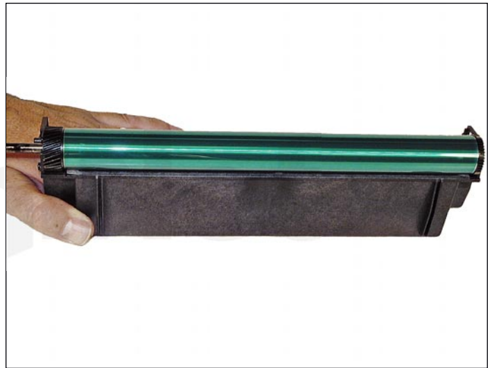
24. Slide the drum axle out from the side opposite the E-ring.
