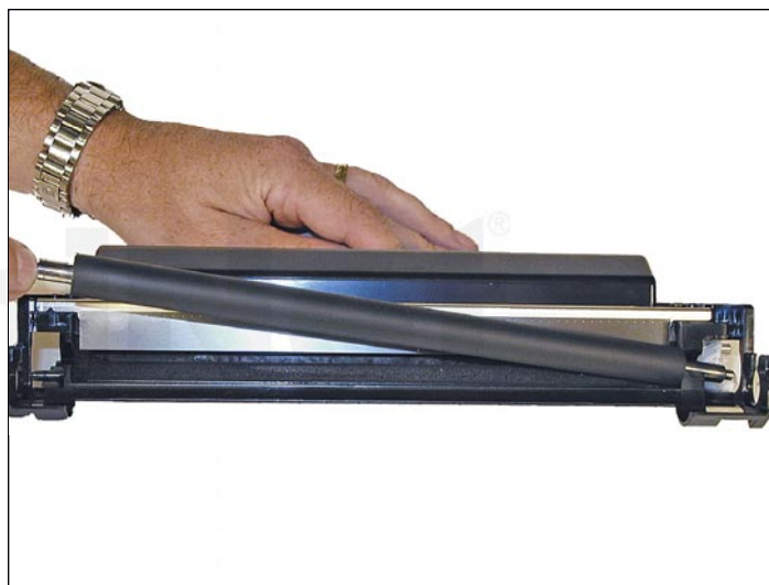
19. Clean and install the developer roller, long shaft side to the gear side first.
