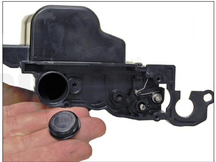
10. On the supply hopper, remove the fill plug and dump out any remaining toner.
