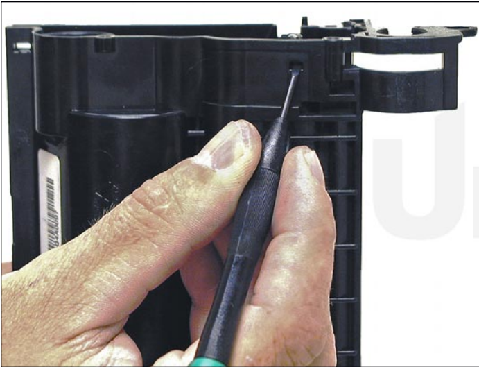
12. On the fill plug side, press in on the plastic tab and remove the spring and plastic bushing assembly.
